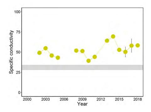
Specific conductivity is a measurement of dissolved solids in water. Regular monitoring helps determine baseline levels. Fluctuations in these levels are an indicator of pollution. The grey shading indicates baseline level of a typical minimially impacted stream in our region.
